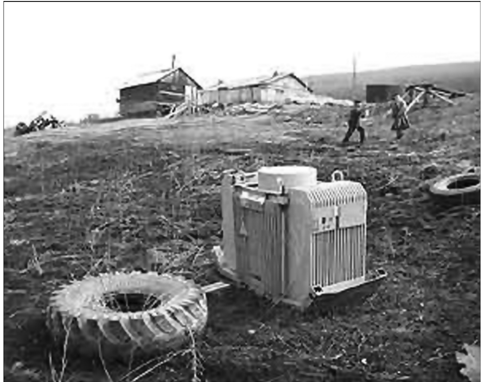
Figure 2: Abandoned Radioisotope Thermoelectric Generator in Russia
